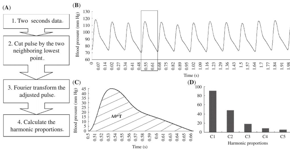
Figure 2. (A) Flowchart of data processing. (B) A typical 2-second pulse sequence data. (C) A typical pulse waveform which was separated by the two neighboring lowest points. (D) A typical harmonic analysis of the pulse waveform.
